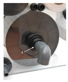
The water outlet may not be reduced. A 40 mm PVC pipe should be presses into the tank union. From here a PVC pipe can be directed to the filter sump or pond. The pipe should not be glued into the tank union. If it is glued, the Rollermat cannot not be disassembled.
