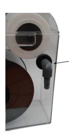
The emergency overflow is a 25 mm tank union. Here, you can press in a 25 mm PVC pipe. From here the pipe is directed downwards in a free flow pipe. Alternatively a 25 mm hose connection can be pressed into the tank union and a hose can be directed to the pond or aquarium.
